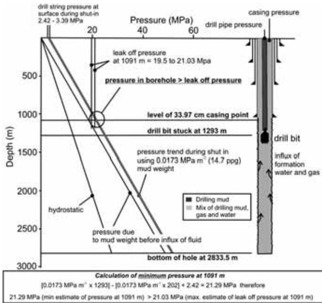
**Fig. 9.** Graph of hydrostatic pressure plotted against depth. The leak off test at 1091 m can be interpreted as between 19.62 MPa (equivalent to 15.9 ppg) and a maximum of 21.03 MPa (equivalent to 16.4 ppg) (vertical grey bar). The pressure in the drill pipe with depth marked by thick black line. Circled region shows that the pressure in the wellbore after the influx of formation fluids would have exceeded the LOT pressure, when the blow out preventors were shut on May 28th 2006.
